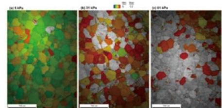
Superposed image quality (IQ) in greyscale and grain orientation spread (GOS) maps of the polished Sn-1.0wt%Bi alloy one hour after polishing under different pressures.
