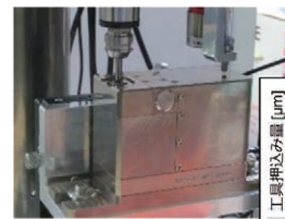
接触式工具長測定器 Contact type tool length measuring system
